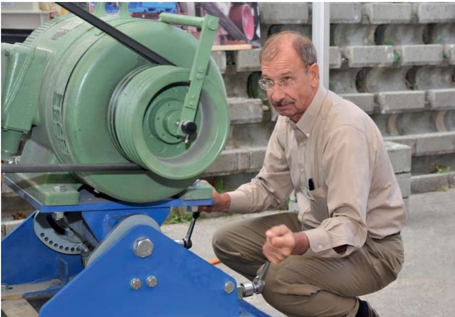
Easy pre-tensioning by means of two pull-out ratchets
