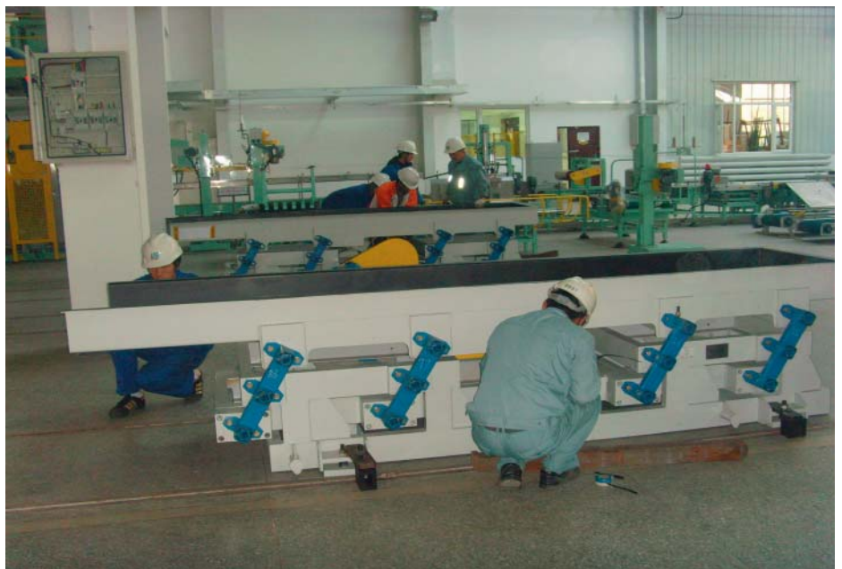
Series production of two-mass oscillating conveyors at Harbin Boshi
