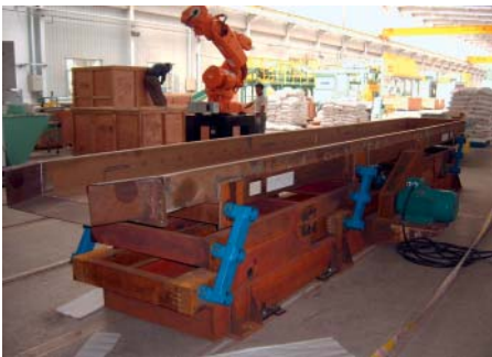
Prototype of the new concept shaker conveyor with AD-P 50 rocker arms
