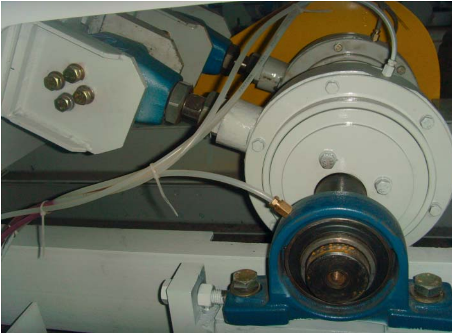
Slider crank drive on the oscillating conveyor with two ROSTA drive heads type ST 50
