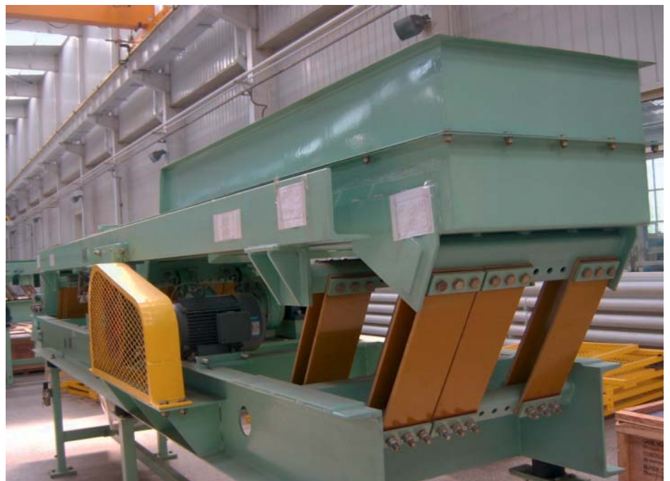
Original oscillating conveyor design with fibreglass slats
